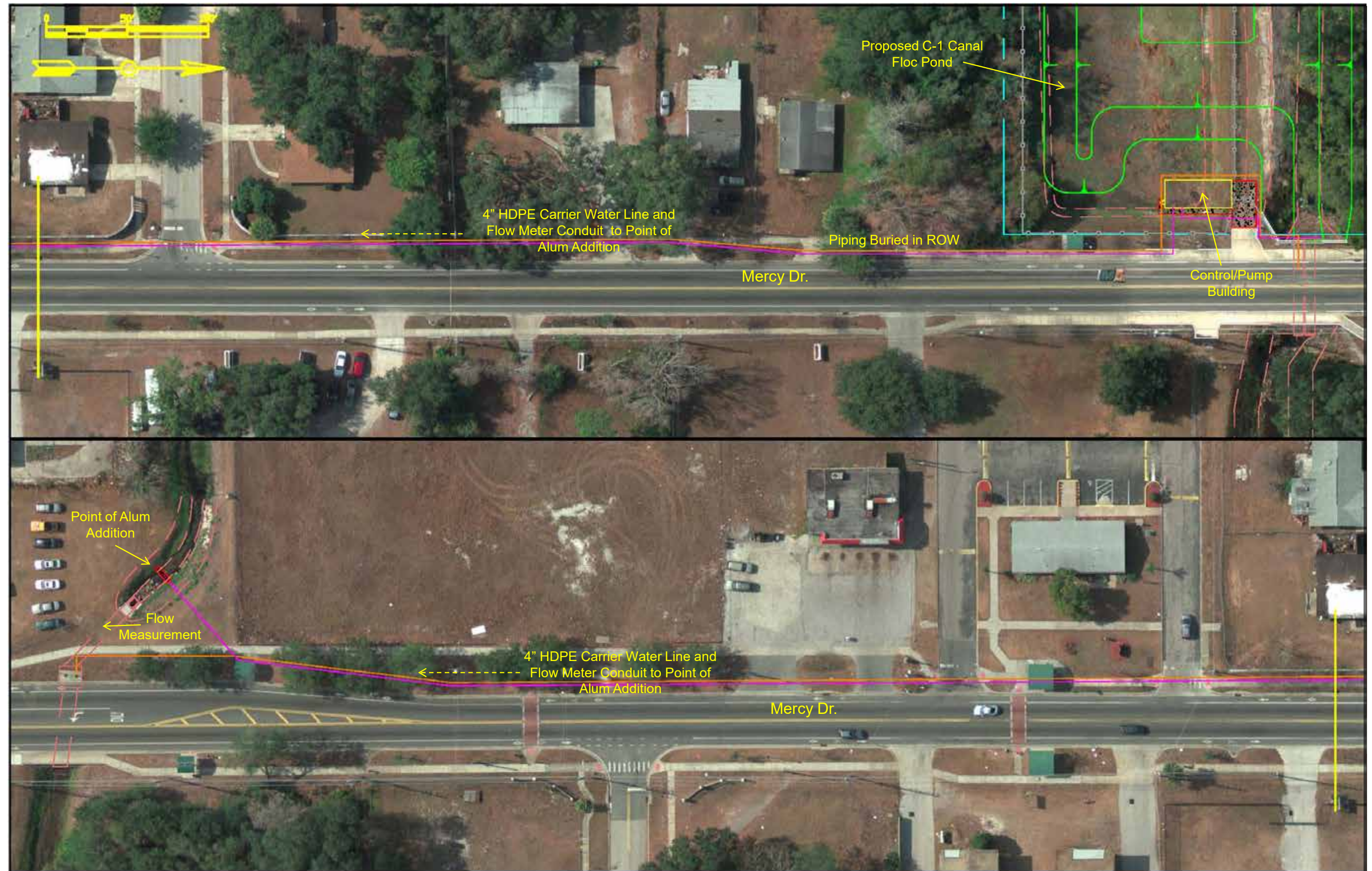
Figure 7-5. Conceptual Design for the Proposed C-2 Canal Alum Treatment System.
