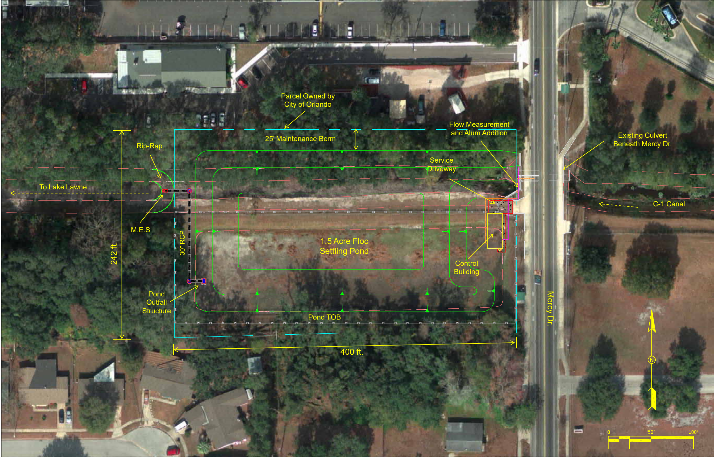
Figure 7-4. Conceptual Design for the Proposed C-1 Canal Alum Treatment System.
