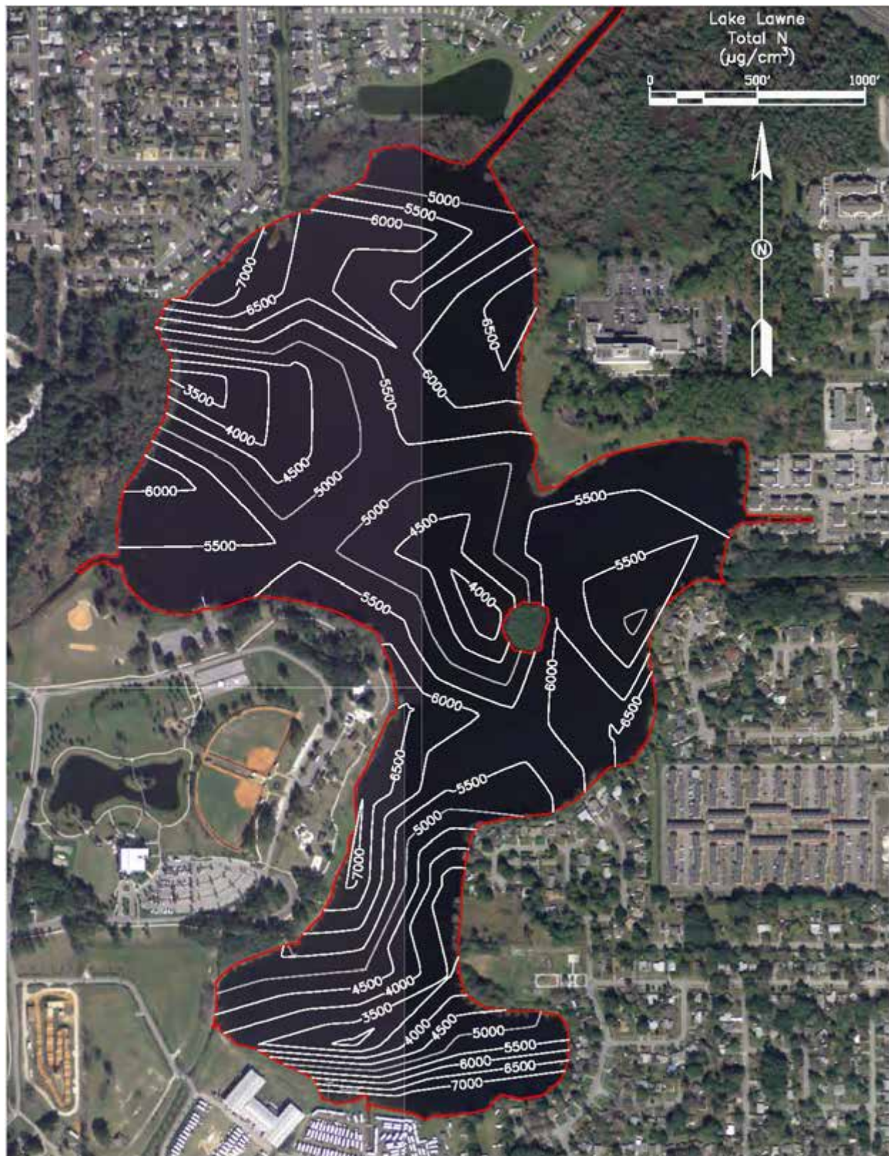
Figure 2-13. Isopleths of Total Nitrogen ( \mu\text{g}/\text{cm}^3 ) in the Top 10 cm of Sediments in Lake Lawne.
