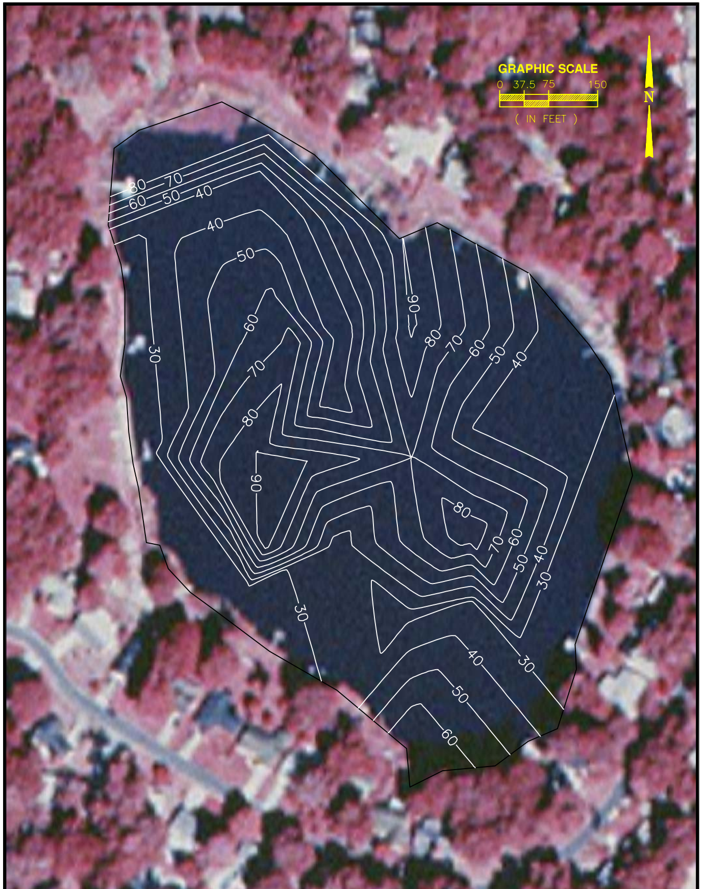
Figure 3-4. Isopleths of Moisture Content (% dry wt.) in the Top 10 cm of Sediments in Lake Anderson.
