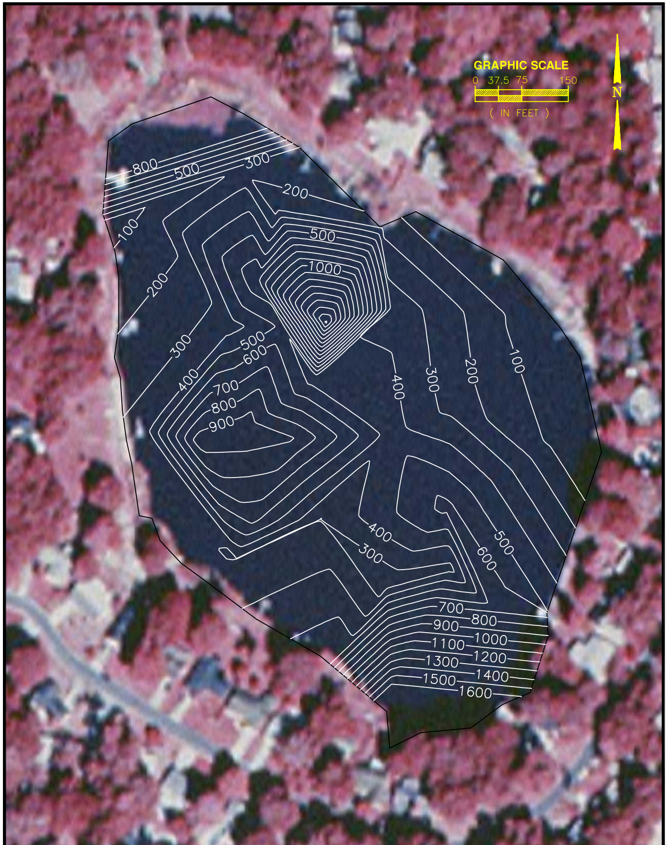
Figure 3-6. Isopleths of Total Phosphorus ( \mu\text{g}/\text{cm}^3 wet wt.) in the Top 10 cm of Sediments in Lake Anderson.
