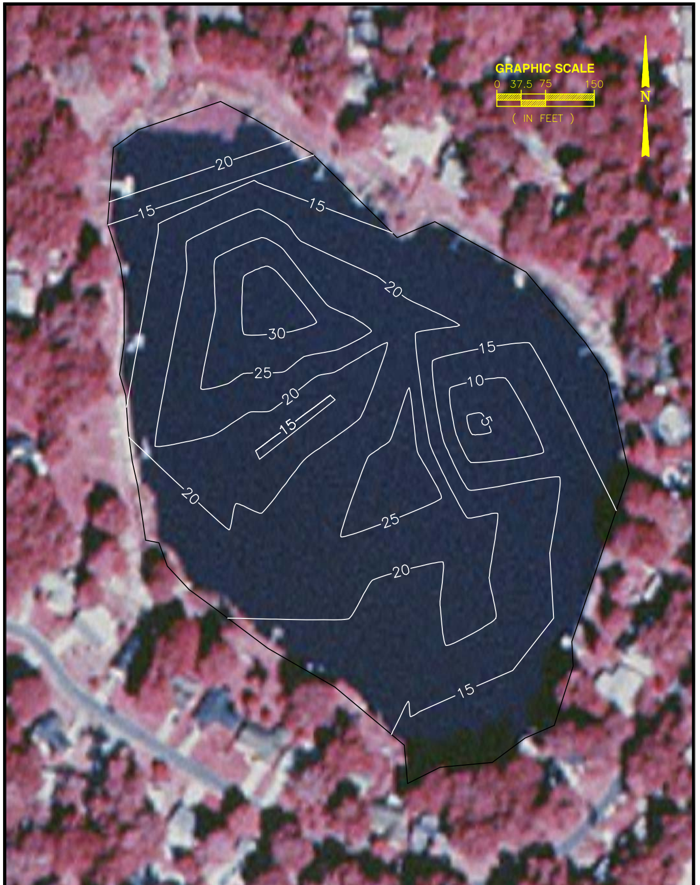
Figure 3-8. Isopleths of Saloid-Bound Phosphorus ( \mu\text{g}/\text{cm}^3 wet wt.) in the Top 10 cm of Sediments in Lake Anderson.
