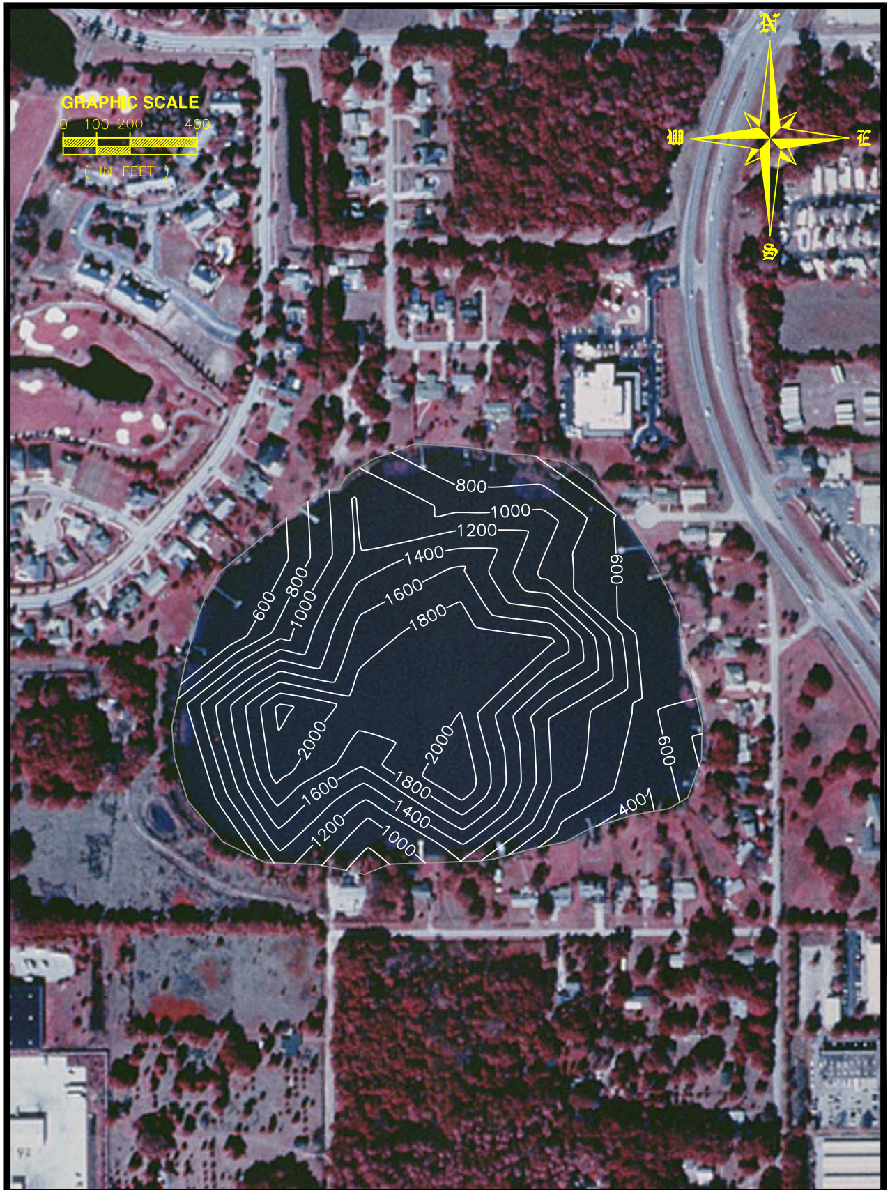
Figure 3-6. Isopleths of Total Phosphorus ( \mu\text{g}/\text{cm}^3 wet wt.) in the Top 10 cm of Sediments in Bay Lake.
