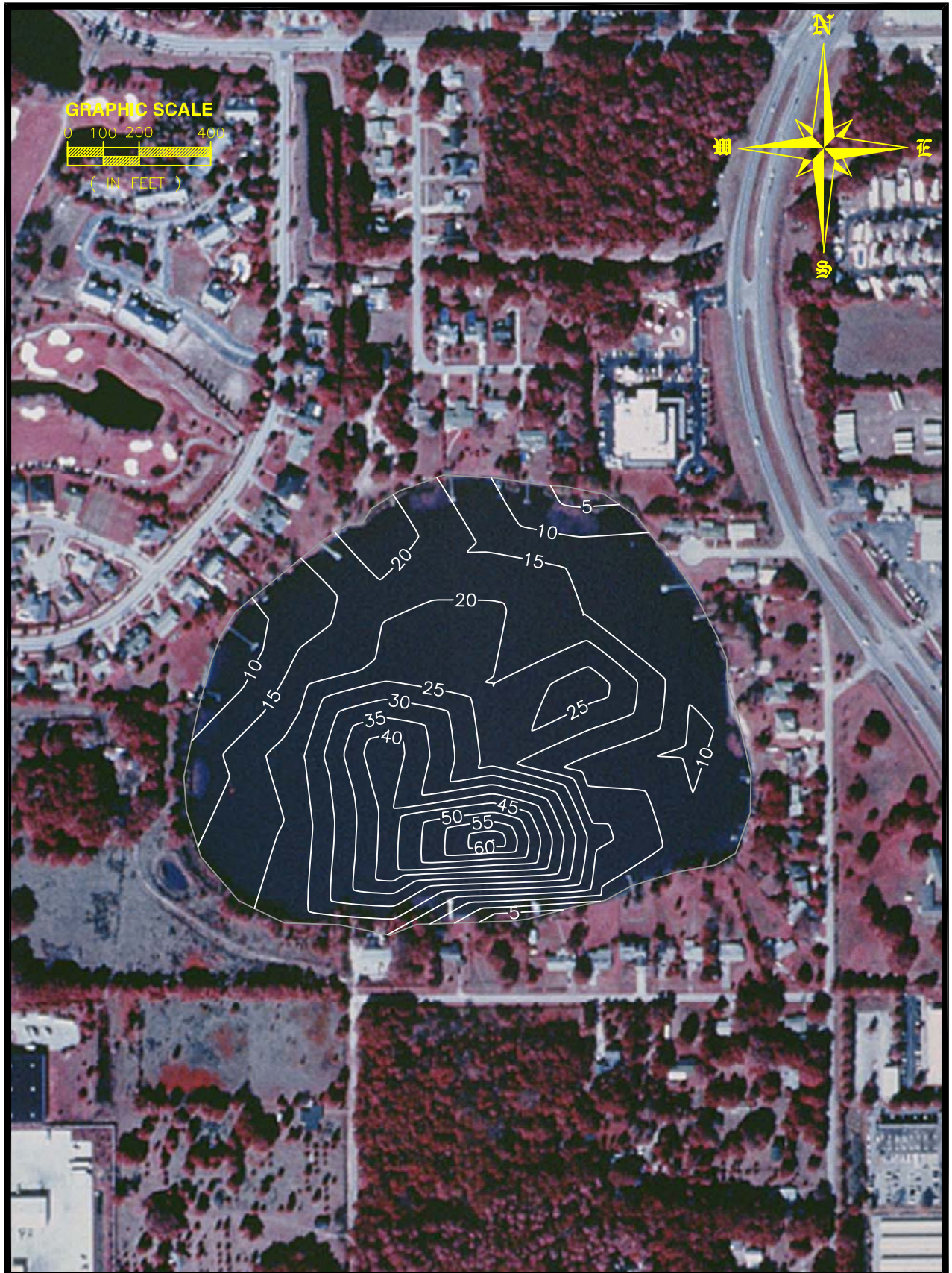
Figure 3-9. Isopleths of Iron-Bound Phosphorus ( \mu\text{g}/\text{cm}^3 wet wt.) in the Top 10 cm of Sediments in Bay Lake.
