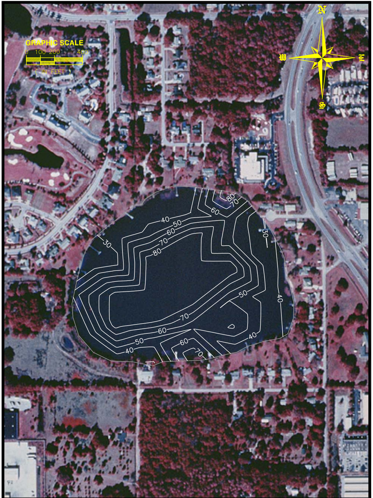
Figure 3-3. Isopleths of Moisture Content (% dry wt.) in the Top 10 cm of Sediments in Bay Lake.
