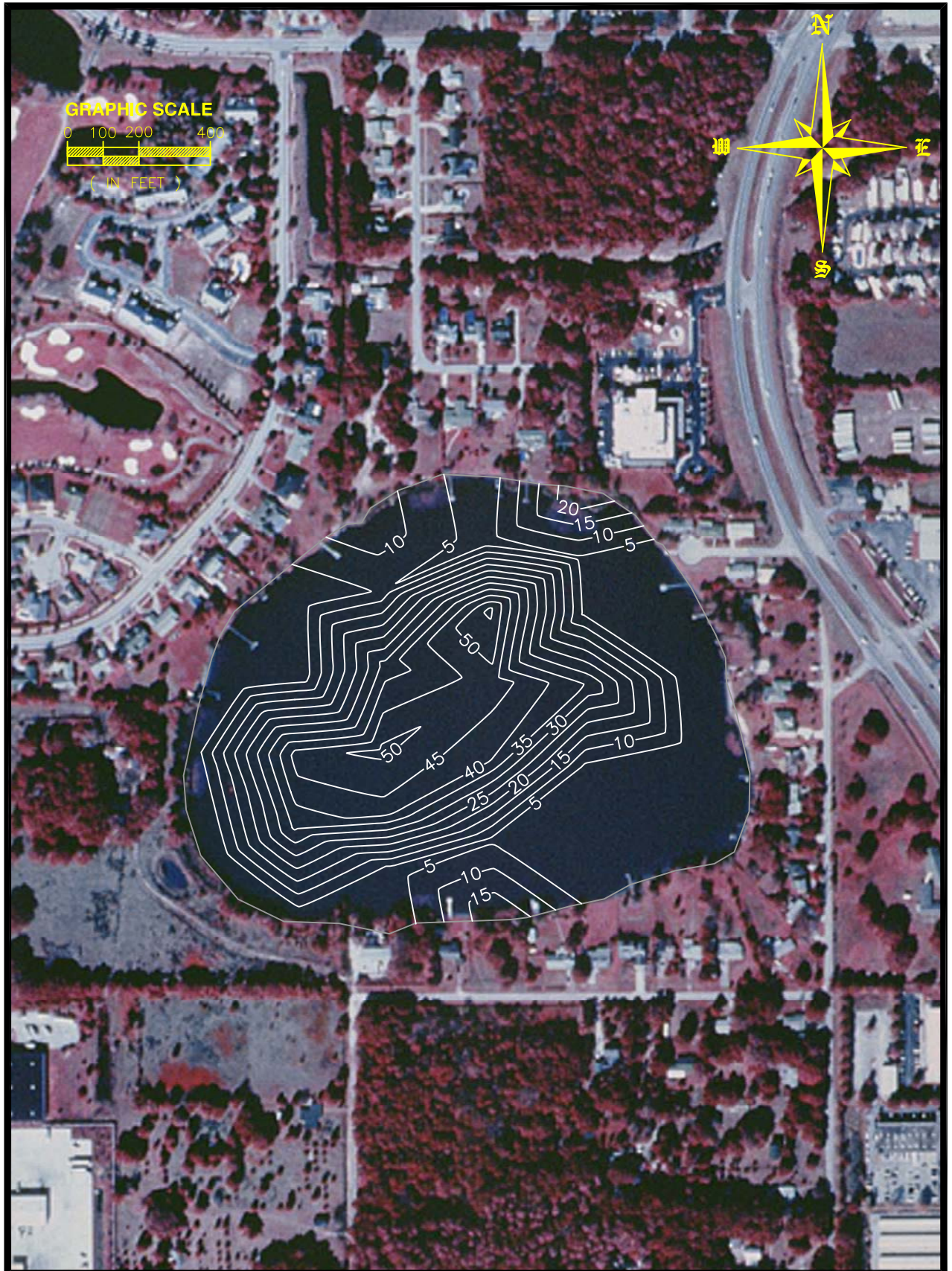
Figure 3-4. Isopleths of Organic Content (% dry wt.) in the Top 10 cm of Sediments in Bay Lake.
