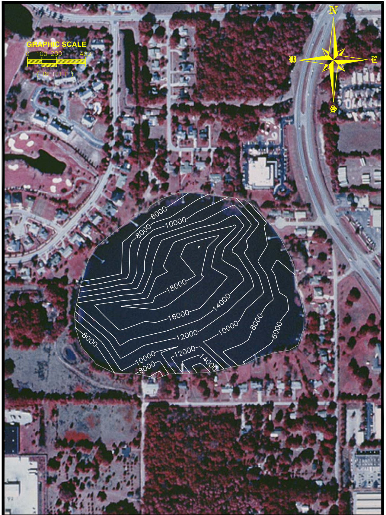
Figure 3-7. Isopleths of Total Nitrogen ( \mu\text{g}/\text{cm}^3 wet wt.) in the Top 10 cm of Sediments in Bay Lake.
