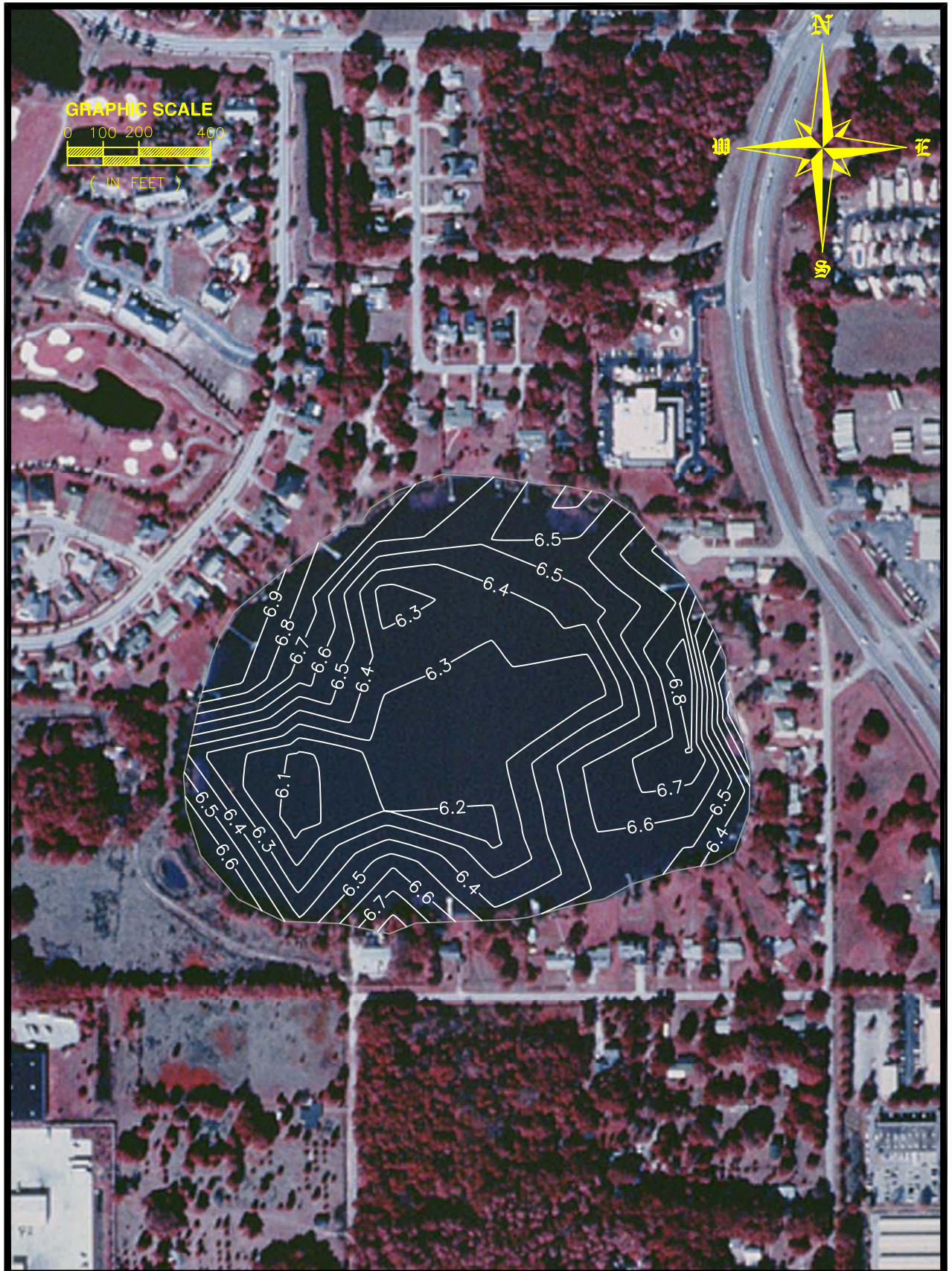
Figure 3-2. Isopleths of pH (s.u.) in the Top 10 cm of Sediments in Bay Lake.
