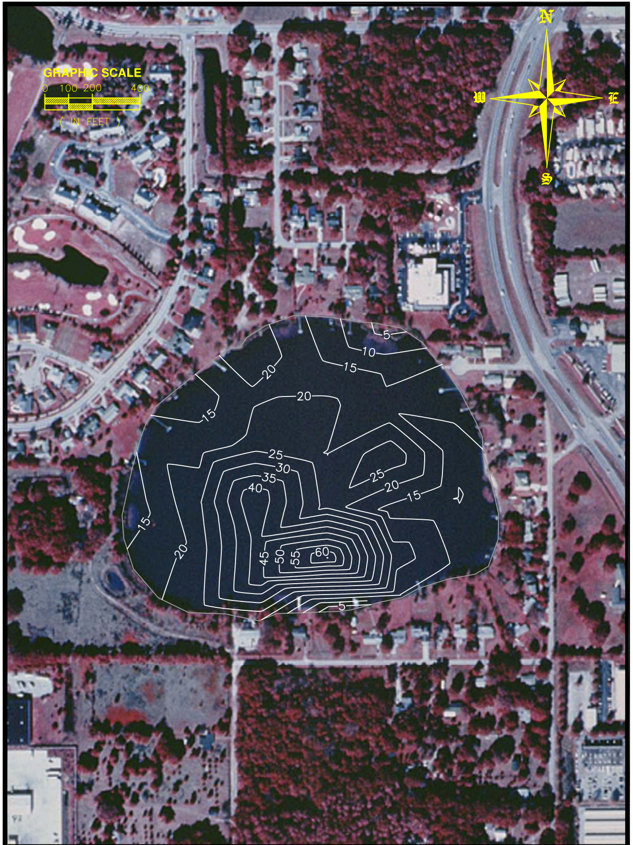
Figure 3-10. Isopleths of Total Available P ( \mu\text{g}/\text{cm}^3 wet wt.) in the Top 10 cm of Sediments in Bay Lake.
