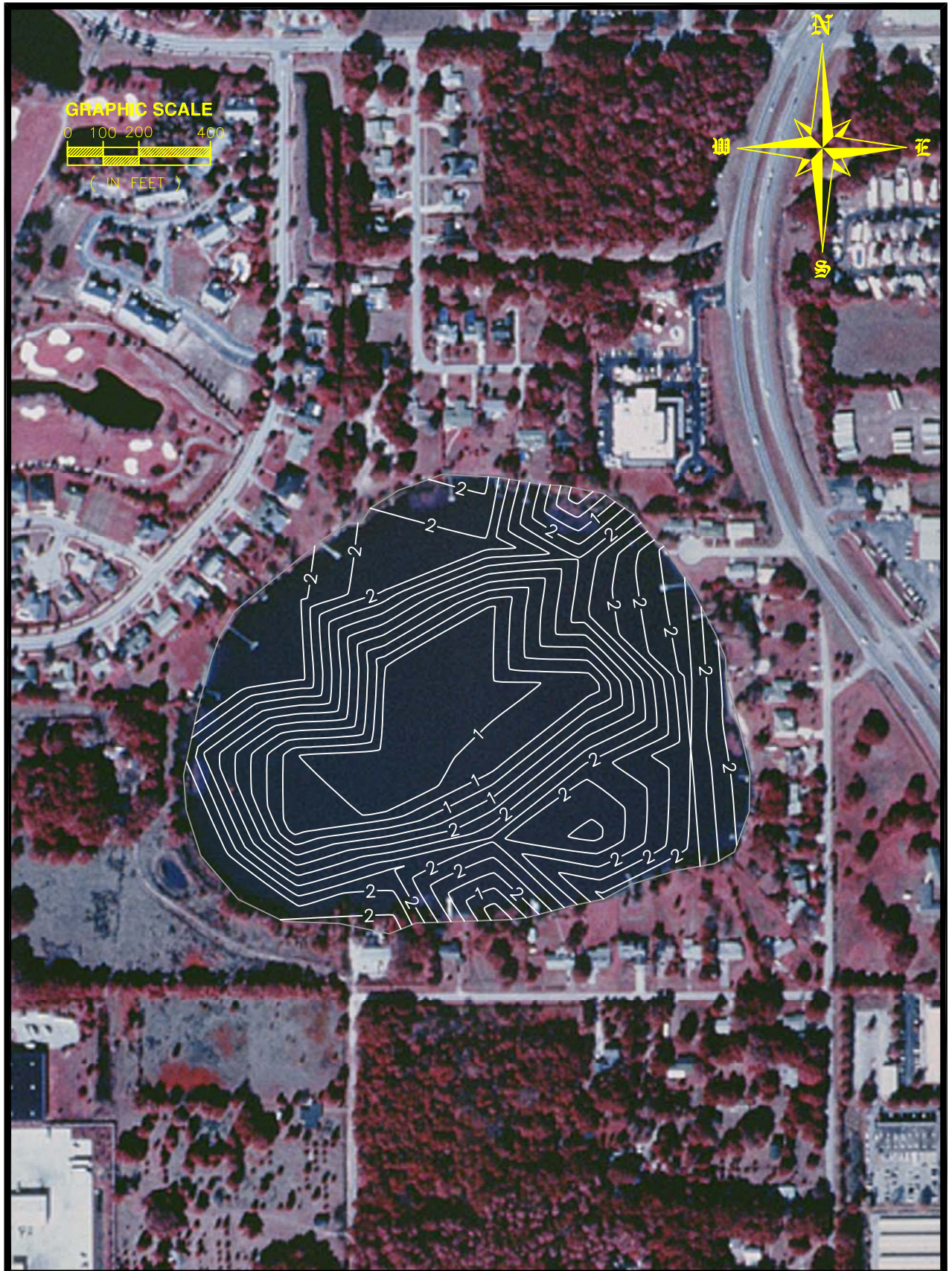
Figure 3-5. Isopleths of Sediment Density ( \text{g}/\text{cm}^3 wet wt.) in Bay Lake.
